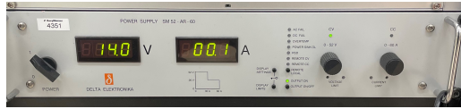
Figure 18: The power supply used to power the BLDC motor is a Delta Elektronika SM 52-AR-60 power supply.
