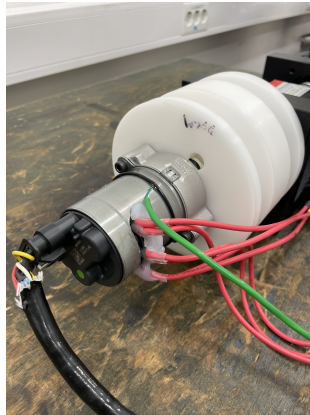
Figure 19: The modified BLDC motor with cables going to and from phases to measure phase currents.
